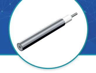
The low-loss semi-rigid cables from Micro-Coax provide lower attenuation, better phase stability with temperature, and a higher operating temperature when compared to traditional solid PTFE semi-rigid cables. This line of semi-rigid cables has 4 available outer conductor options: copper, tin-plated copper, aluminum, or tin-plated aluminum.
