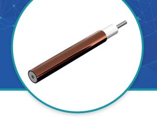
The low-loss semi-rigid cables from Micro-Coax provide lower attenuation, better phase stability with temperature, and a higher operating temperature when compared to traditional solid PTFE semi-rigid cables. This line of semi-rigid cables has 4 available outer conductor options: copper, tin-plated copper, aluminum, or tin-plated aluminum.
